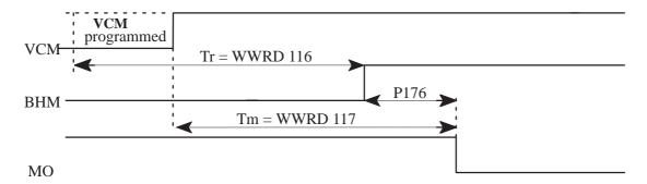
Tr = robot disengaging time in 1/10 s (WWRD 116)
